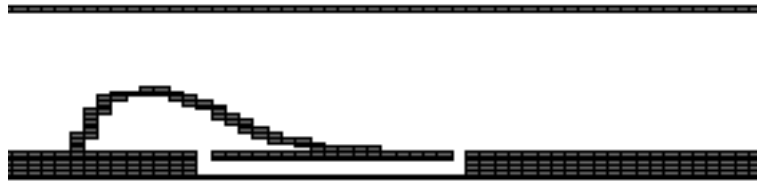
Figure 2.3: A pipe is created in the model of Hamburg to prevent the enclosure of air.
