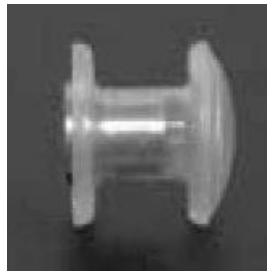
Figure 4.1: The shunt valve with inside the cylindrical metal housing.
