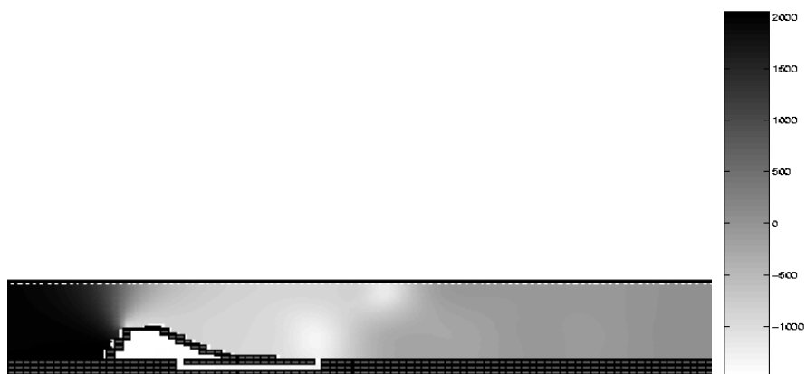
The pressure distribution when the lip is still in contact with the lower wall.
