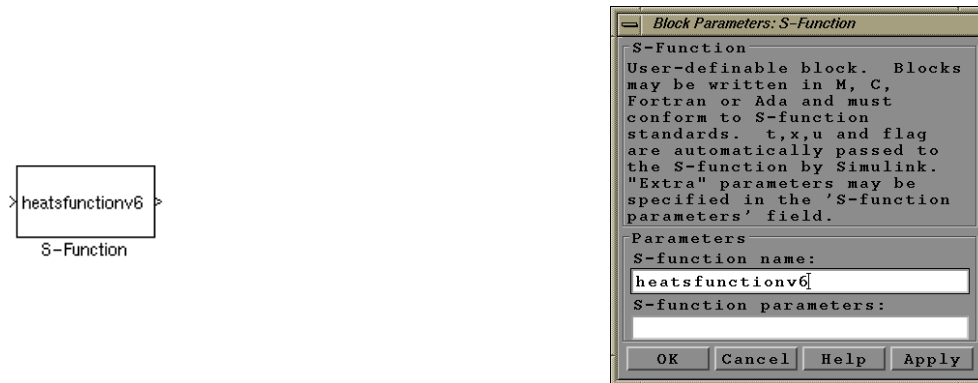
Figure A.2: S-function block with parameters.
