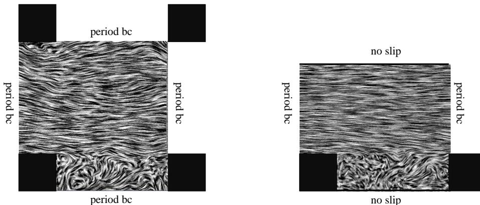
Figure 1: Top- and side-view of a sub-channel unit. Both pictures show an instantaneous flow field (taken from the DNS) at the plane that bisects the cubes. The flow is directed from left to right.
