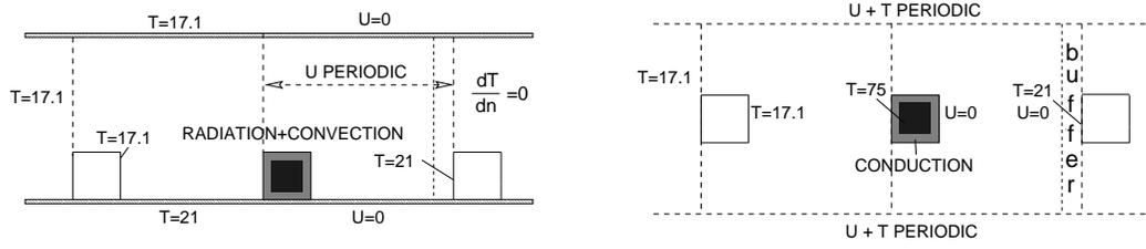
Figure 2: An overview of the boundary conditions. The left hand side picture shows a side-view of the channel; the right hand side displays a top-view.
