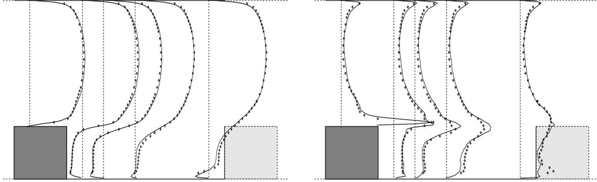
Figure 6: A comparison of first-order statistics (left handside picture) and second-order statistics (right handside) of the DNS with experimental data. Shown are the mean streamwise velocity  $\bar{u}$  (left) and  $\overline{u'u'}$  (right) in the plane parallel to the streamwise direction that bisects the cubes. The continuous lines correspond to the DNS; the experimental data is depicted by the dots.
