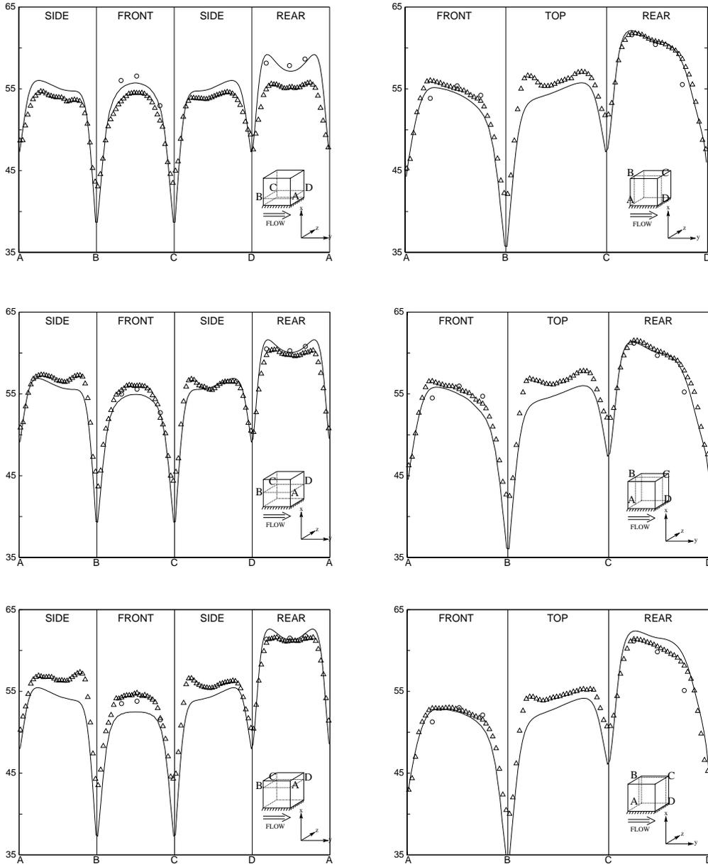
Figure 7: The mean temperature along different paths at the surface of the heated cube. The markers denote the experimental data by Meinders *et al.* Note that at three points along BC and DA (left-hand column) and at three points along AB and CD (right-hand column) two data-points are available. Both are shown.
