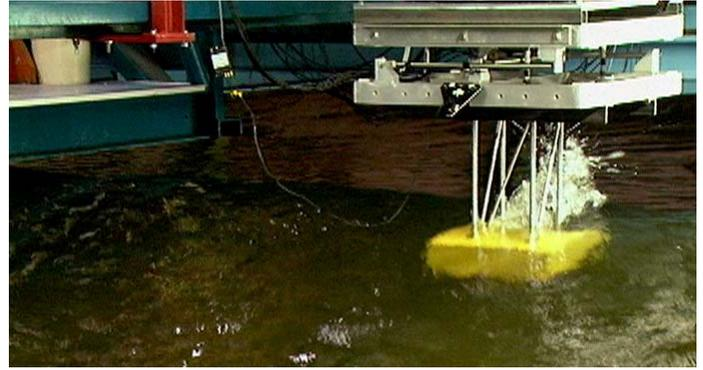
Figure 4: Captive block in focused wave test.
