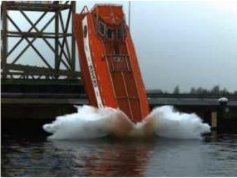
Fig. 1 Drop test with free-fall lifeboat (from: www.verhoef.eu)
