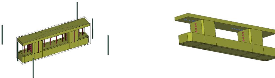
Figure 12: Positions of the sensors for surface elevation (left) and pressure (right).
