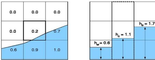
Fig. 3: Construction of the LHF around a central S-cell by summing  $F_S$  values vertically.
