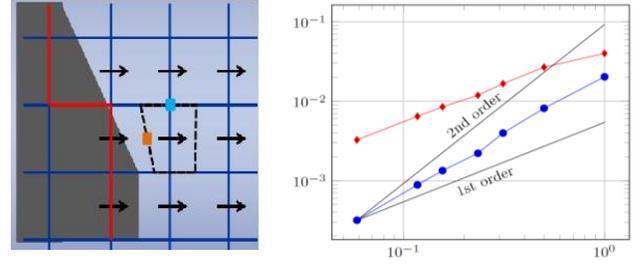
Fig. 9: Left: the LSSTAG discretisation of momentum diffusion is based on the deformed momentum control volume (dashed region), making careful use of aperture information. Right: difference between numerical and analytical velocity ( $L_2$ -norm) for Hagen-Poiseuille flow; with (red) and without (blue) improved discretisation of diffusion.
