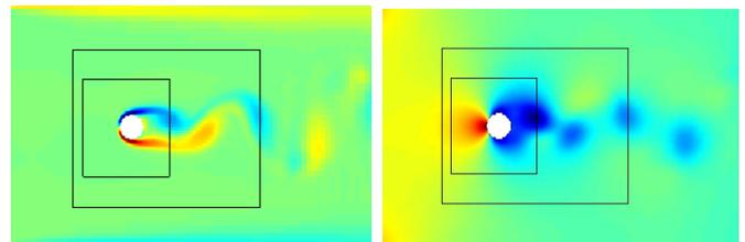
Fig. 12: Computed pressure distribution (left) and vorticity (right) for the flow around a circular cylinder ( $D=1m$ ,  $U_{in}=1$  m/s,  $Re = 100$ ). The flow goes through the refinement layers without visual disturbance.
