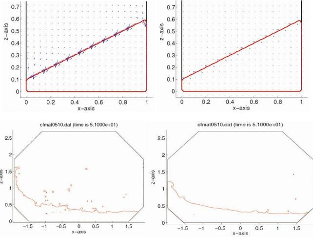
Fig. 6: Top row: hydrostatic case, with gravity  $\mathbf{g} = (1, -2)$  perpendicular to the oblique free surface. Bottom row: liquid configuration after two simulations of a regular sway sloshing experiment. With sophisticated gravity-consistent density averaging (right) much less instabilities are observed than with simple geometrical averaging (left).
