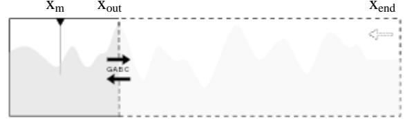
Fig. 7: The two domains used to test the performance of the ABC. A short domain, with either Sommerfeld or ABC imposed at  $x_{out}$ , and the long domain with boundary at  $x_{end}$ . Reflections at  $x_m$  are measured from the difference between long and short domains.
