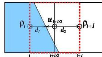
Fig. 5: The gravity-consistent density average  $\rho_{i+1/2}$  is found by weighting  $\rho_i$  and  $\rho_{i+1}$  with the fraction (coefficients  $d_1$  and  $d_2$ ) that the free surface splits the red-dashed momentum control volume.
