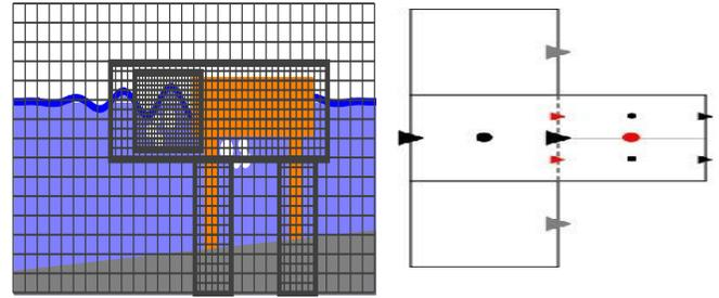
Fig. 11: LGR in the simulation of a wave around an offshore structure (left). Discretisation near the refinement involves known (black/grey) and virtual variables (red); cells are split with a 1:2 ratio (right).
