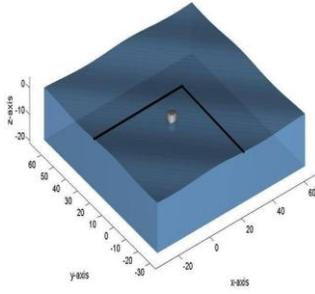
Fig. 8: For waves entering the domain under an angle  $\alpha$ , outflow boundaries can be taken close to the structure, at both x- and y-planes, which saves computing time significantly.
