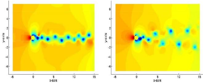
Fig. 10: Snapshots of the pressure field during vortex shedding behind a circular cylinder ( $Re=2000$ ), with pure central discretisation (left) and central discretisation with  $C_2$  regularisation (right).
