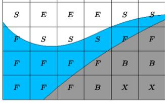
Fig. 2: Example (2D) of cell labeling: dark shading represents solid, blue and white represent water and air, respectively.
