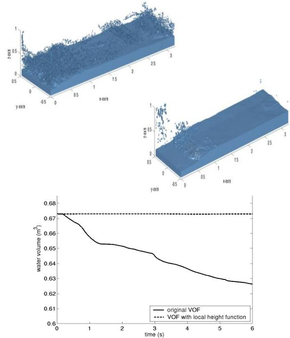
Fig. 4: The use of LHF (middle) results in significantly less erroneous droplets, compared to the original SLIC/VOF method (top), and is perfectly mass-conserving (bottom).
