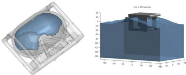
Fig. 13: Examples of IBM studies with ComFLOW: Sloshtat FLEVO (left) and Statoil Snorre TLP (right).
