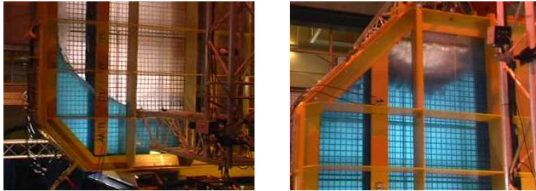
Figure 1: Screenshots of the 10 percent (left) and 95 percent (right) filling ratio sloshing model experiment.
