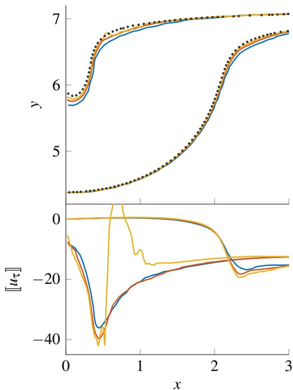
**Figure 7:** Interface profiles (top) and velocity discontinuity (bottom) for  $\rho^g = 1 \text{ kg/m}^3$  at two time-instances  $t = 1.47, 1.67$ . Refinement levels are  $l = 2$  (blue), 3 (red) and 4 (yellow). Reference solution by CADYF (black markers) [1].
