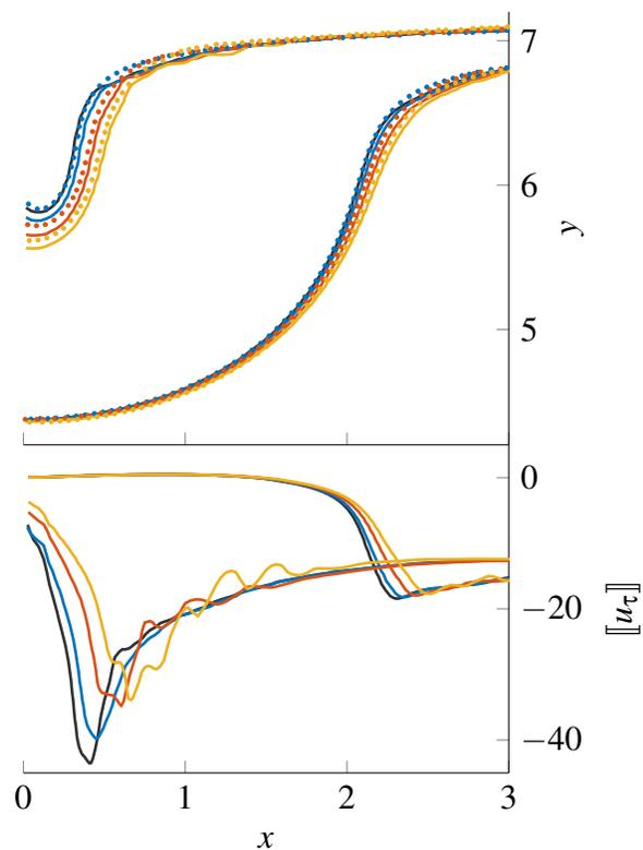
**Figure 8:** Interface profiles (top) and velocity discontinuity (bottom) for gas densities  $\rho^g = 10^{-3}$  (black), 1 (blue), 3 (red) and  $5 \text{ kg/m}^3$  (yellow) at  $t = 1.47, 1.67$ . The refinement level was  $l = 3$ . Reference solutions by CADYF (colored markers) [1].
