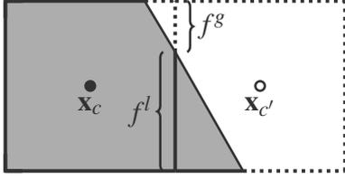
**Figure 1:** Illustration of the CCM. Each face is split into its liquid and gaseous part  $f = f^l \cup f^g$ . Shaded region corresponds to the liquid parts  $c^l, c'^l$ . Solid nodes correspond to the liquid phase and open nodes to the gas phase.
