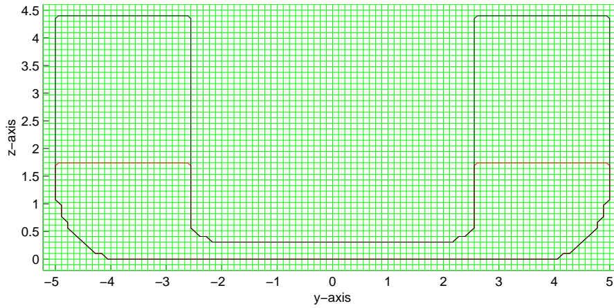
Figure 4.3: Geometry and 100x44 grid used with the simulations
