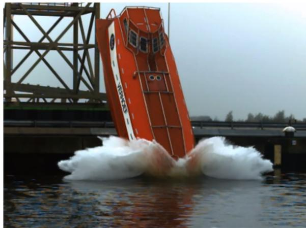
**Figure 1:** Drop test with free-fall lifeboat (from: [www.verhoef.eu](http://www.verhoef.eu))
