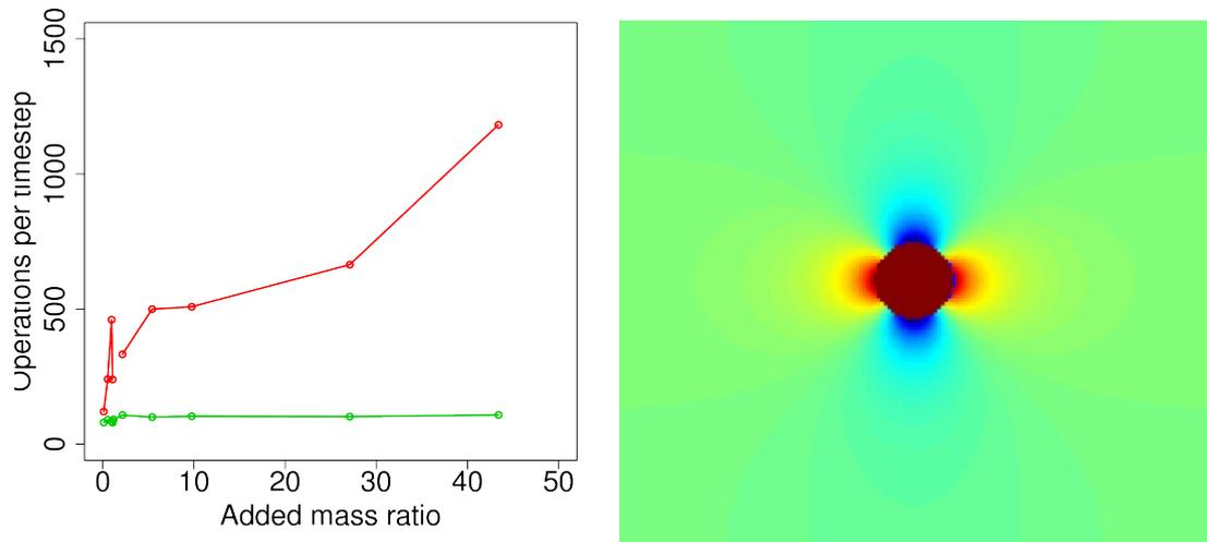
Fig. 4: Total number of matrix-vector products per timestep against added mass ratio of a submerged cylinder. Original method shown in red, the current modified method shown in green.
