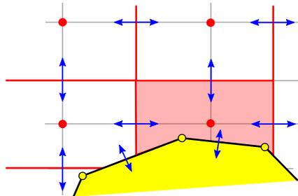
Fig. 3: Finite volume discretization on a staggered grid with cut cells. The solid is shown in yellow, pressures (and associated cells) in red, velocities in blue.
