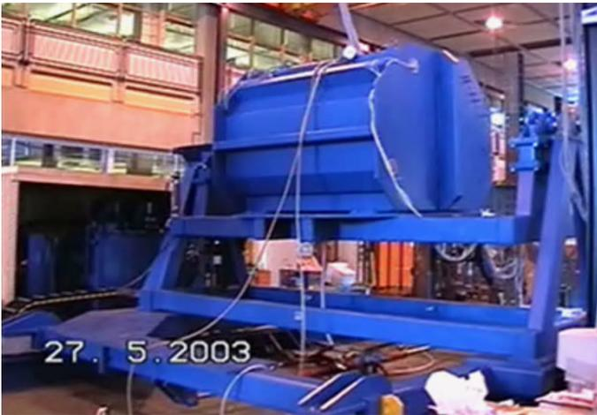
**Figure 11: The LNG tank model**
