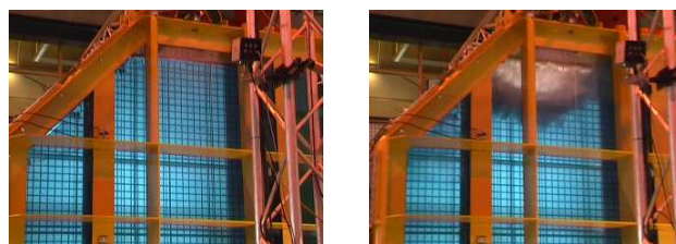
Figure 11. Screenshots of the 95 percent filling-ratio sloshing model experiment. The left picture shows the fluid configuration at t = 0s , the right picture the configuration at t = 8.8s .
