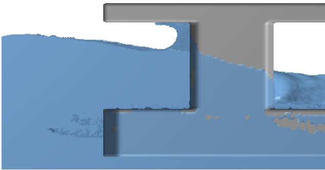
Figure 16. Long wave, the 1<sup>st</sup> column run-up, stage (b)
