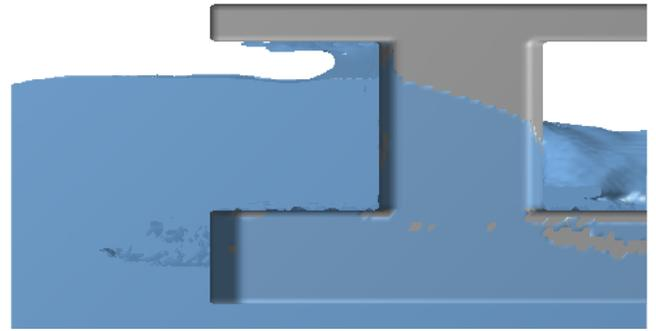
Figure 17. Long wave, the 1<sup>st</sup> column run-up, stage (c)
