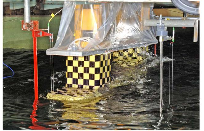
Figure 1. Experimental model, semi-submersible
