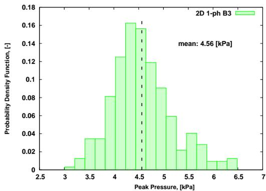
Figure 22. Binned pressure peaks, 2D calculation
