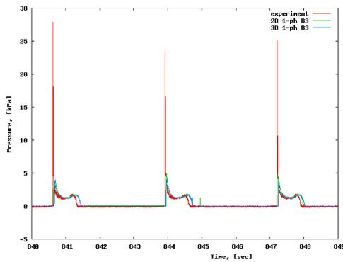
Figure 8. Experimental and computational records,  $t=840-849$  [sec]
