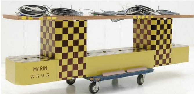
(a) THE 1:50 MODEL OF THE SEMI-SUBMERSIBLE IN THE WORK SHOP.
