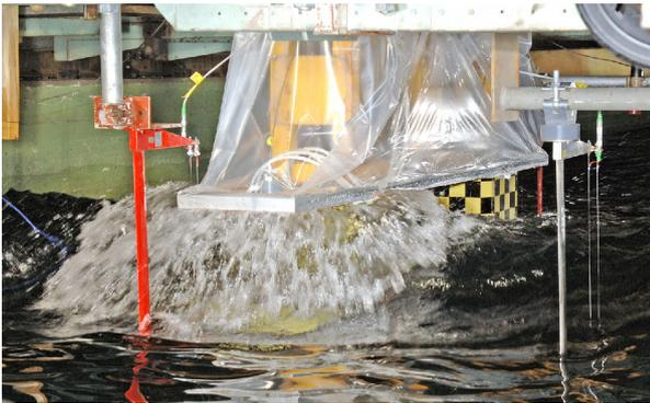
(b) WAVE RUN-UP AND IMPACT ON THE FORWARD COLUMN AND DECK IN REGULAR WAVES.
