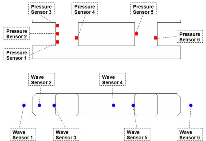
(b) POSITIONS OF THE WAVE PROBES AND PRESSURE TRANSDUCERS.
