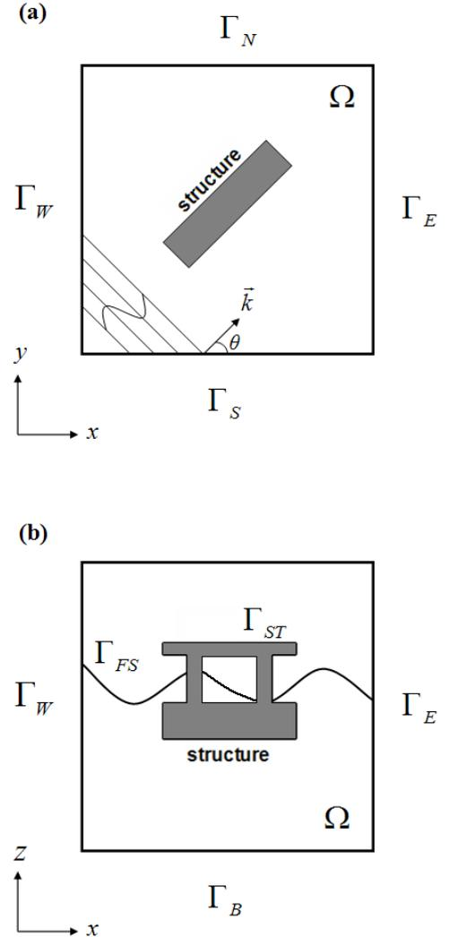
**FIGURE 1.** A COMPUTATIONAL DOMAIN WITH A STRUCTURE LOCATED AT THE CENTER.  $\Gamma_N$ ,  $\Gamma_E$ ,  $\Gamma_S$  and  $\Gamma_W$  ARE ARTIFICIAL BOUNDARIES ON WHICH AN ABC IS TO BE APPLIED.
