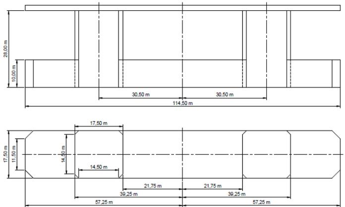
(a) GENERAL PLAN OF THE SEMI-SUBMERSIBLE AT FULL SCALE.
