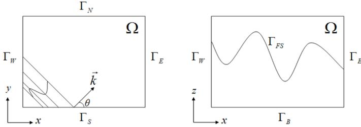
**FIGURE 1.** A COMPUTATIONAL DOMAIN WITH  $\Gamma_N$  AND  $\Gamma_E$  AS ARTIFICIAL BOUNDARIES.
