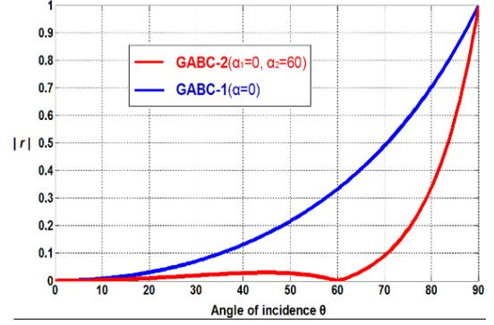
**FIGURE 3.** REFLECTION COEFFICIENTS FOR ABC-1 ( $\alpha = 0$ ) vs ABC-2 ( $\alpha_1 = 0$ ,  $\alpha_2 = 60^\circ$ ) FOR A GIVEN WAVE SPEED AS A FUNCTION OF THE ANGLE OF INCIDENCE.
