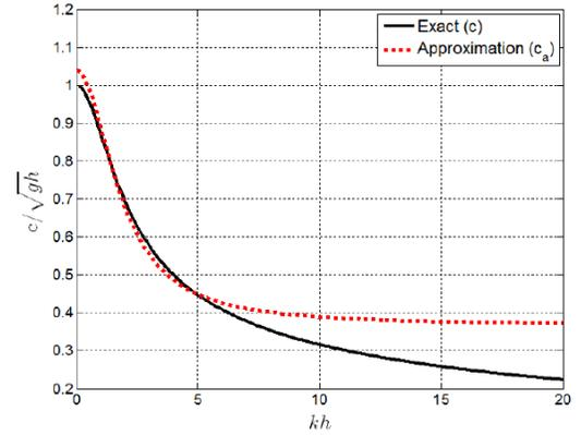
**FIGURE 2.** APPROXIMATION OF THE DISPERSION RELATION. FOR THE COEFFICIENTS IN (11),  $a_0 = 1.04$ ,  $a_1 = 0.106$  AND  $b_1 = 0.289$  ARE USED.
