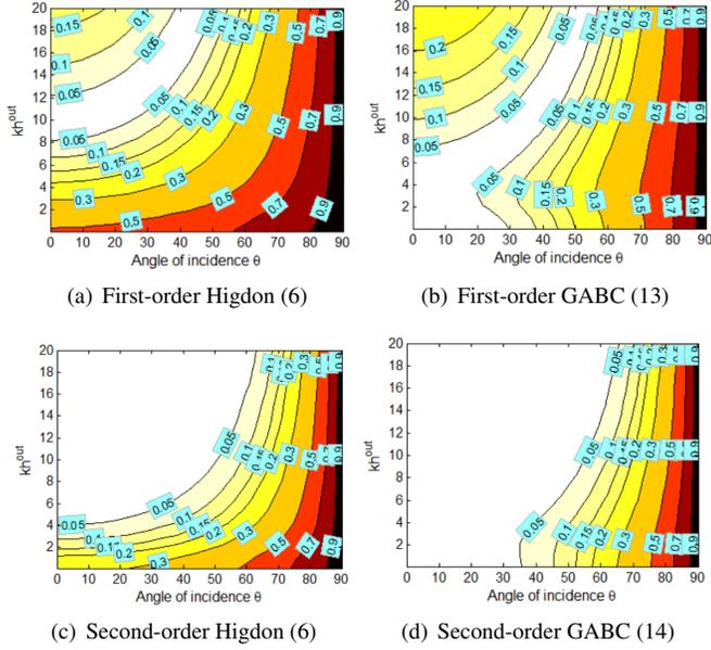
**FIGURE 4.** AMOUNT OF REFLECTION (IN PERCENT) AS A FUNCTION OF THE ANGLE OF INCIDENCE  $\theta$  AND  $kh$  WHEN VARIOUS BOUNDARY CONDITIONS ARE USED. REFLECTION VALUES ARE WRITTEN ON THE CONTOUR LINES.
