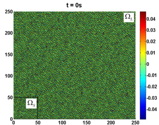
FIGURE 7. THE SETUP FOR THE DIRECTIONAL IRREGULAR WAVE SIMULATION.
