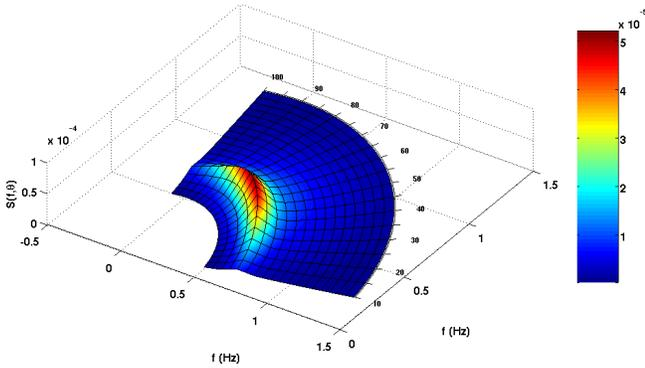
**FIGURE 9.** THE DIRECTIONAL SPECTRUM OF THE IRREGULAR WAVE.
