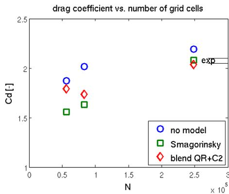
**FIGURE 3.** COMPUTED DRAG COEFFICIENT FOR FLOW PAST A SQUARE CYLINDER AT  $Re = 22,000$  FOR SEVERAL TURBULENCE MODELS AND NUMBER OF GRID POINTS ( $N$ ).
