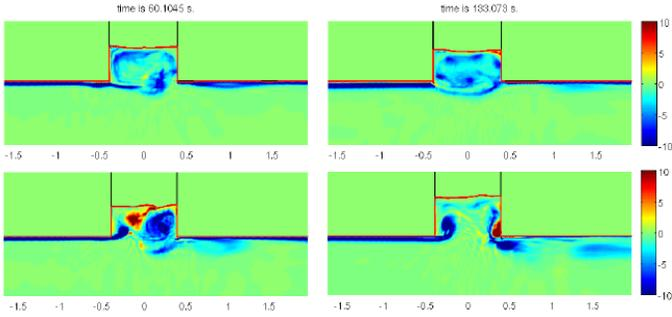
**FIGURE 5.** DEVELOPMENT OF VORTICITY IN TIME (FROM LEFT TO RIGHT: 60 s AND 133 s) FOR A FINAL SPEED (AFTER ACCELERATION) OF 0.7 m/s (TOP) AND 1.0 m/s (BOTTOM).
