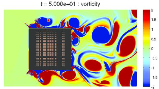
**FIGURE 1.** SNAPSHOT ON A FINE GRID AT  $t = 50s$  OF THE VORTICES CLOSE TO THE CYLINDER; GIVING AN IMPRESSION OF THE SMALL LENGTH SCALES PRESENT IN THE FLOW.
