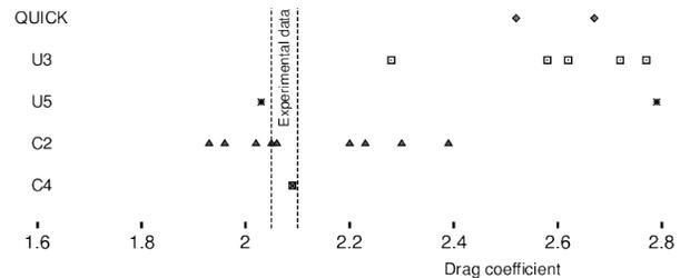
**FIGURE 2.** THE MEAN DRAG COEFFICIENT FOR FLOW PAST A SQUARE CYLINDER AT  $Re = 22,000$  FOR VARIOUS LES-MODELS ORDERED BY THE DISCRETIZATION OF THE CONVECTIVE TERM (STATUS IN 1997).
