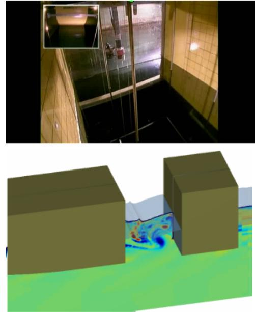
**FIGURE 4.** TOP: PHOTOGRAPH OF THE MOONPOOL EXPERIMENT. BOTTOM: SNAPSHOT OF THE SIMULATION SHOWING VORTEX SHEDDING.
