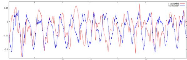
**FIGURE 8.** EXPERIMENT vs SIMULATION: PART OF A TIME TRACE OF THE WATER HEIGHT IN THE MIDDLE OF THE MOONPOOL AS A FUNCTION OF TIME. NOTE THAT THE AMPLITUDES ARE QUITE COMPARABLE.
