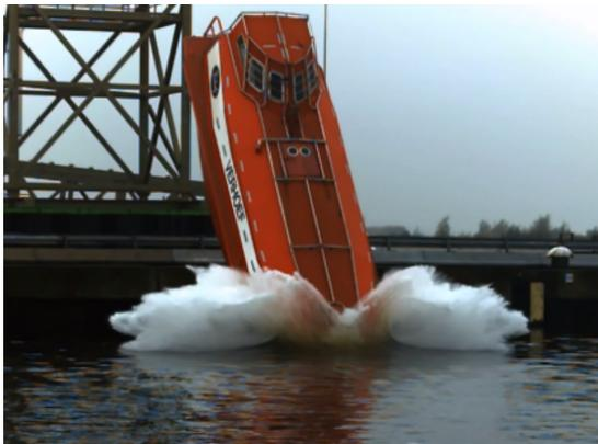
**FIGURE 1.** DROP TEST WITH FREE-FALL LIFEBOAT (FROM: WWW.VERHOEF.EU)
