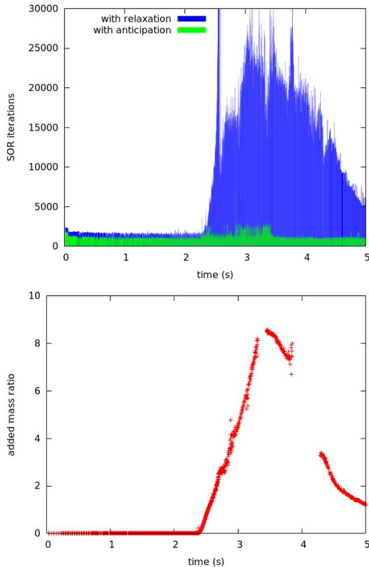
**FIGURE 5.** *TOP:* THE NUMBER OF SOR ITERATIONS PER TIME STEP FOR THE UNDERRELAXED WEAK COUPLING METHOD (BLUE) AND THE ANTICIPATORY QUASI-SIMULTANEOUS METHOD (GREEN). *BOTTOM:* THE ESTIMATED ADDED MASS FOR THE FALLING LIFEBOAT AS A FUNCTION OF TIME. THE CROSSING OF THE FREE SURFACE IS CLEARLY VISIBLE IN THE ADDED MASS.
