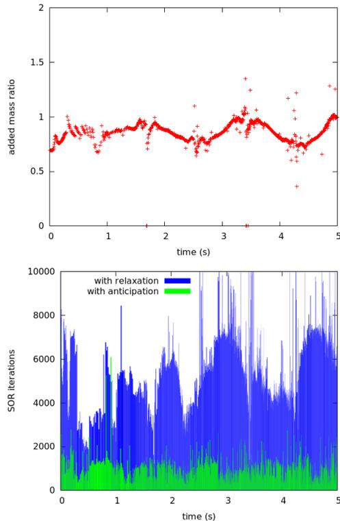
**FIGURE 7.** WORKLOAD OF THE SIMULATION OF A TENSION-LEG PLATFORM IN A STOKES-5 WAVE. *TOP:* VARIATION OF THE EFFECTIVE ADDED-MASS RATIO OVER TIME. *BOTTOM:* THE WORKLOAD FOR THE SIMULATION CORRESPONDS TO THE AREA UNDER THE CURVE.
