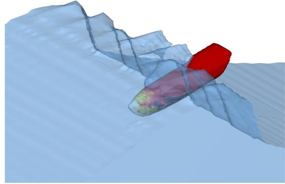
**FIGURE 4.** A SIMULATION SNAPSHOT OF THE LIFE BOAT FALLING INTO A LARGE WAVE.
