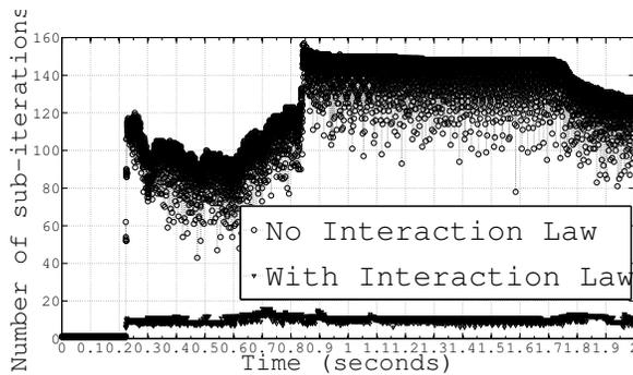
**FIGURE 11.** COMPARISON BETWEEN NUMBER OF SUB-ITERATIONS AT EACH TIME STEP FOR CONVENTIONAL METHOD WITH NO INTERACTION LAW WITH RELAXATION OF 0.05 AND THE NEW METHOD WITH THE INTERACTION LAW WITH RELAXATION OF 0.50
