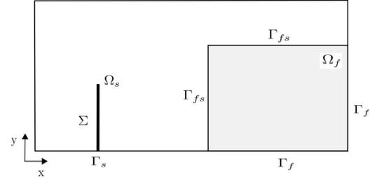
FIGURE 1. SKETCH OF FLUID AND STRUCTURE DOMAIN.
