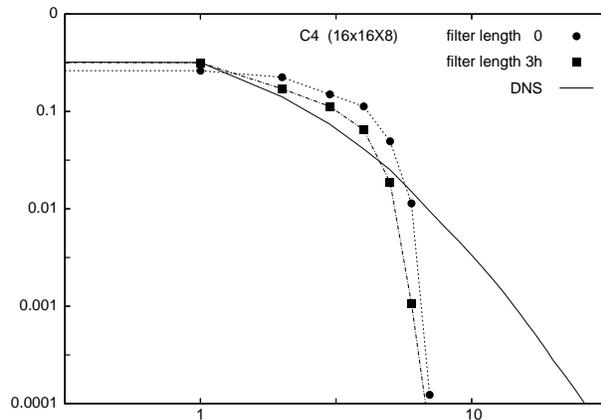
Figure 6: One-dimensional (streamwise) energy spectrum at  $y^+ \approx 5$ , i.e. at the first grid point of the  $16 \times 16 \times 8$  grid.
