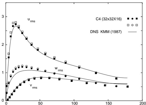
Figure 5: Rms velocity fluctuations;  $32 \times 32 \times 16$  grid points. The open boxes and circles correspond with  $\epsilon = h$ ; the filled boxes and circles represent data that is extrapolated to  $\epsilon = 0$ .
