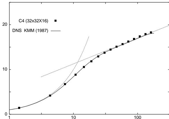
Figure 4: The mean velocity (in wall coordinates) of the  $32 \times 32 \times 16$  simulations for  $\epsilon = h$ .
