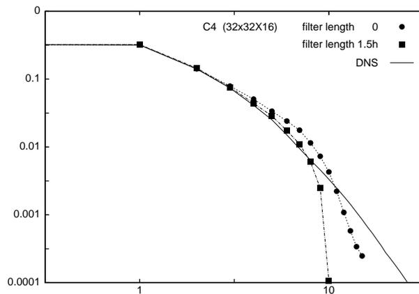
Figure 7: One-dimensional (streamwise) energy spectrum at  $y^+ \approx 5$ ;  $32 \times 32 \times 16$  grid points. The smoothing improves the low modes, whereas the high modes vanish faster.
