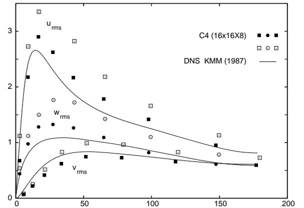
Figure 3: The root-mean-square velocity fluctuations ( $C_4$ ;  $16 \times 16 \times 8$  grid points). The open boxes and circles correspond with  $\epsilon = 2.5h$ ; the filled boxes and circles represent data that is extrapolated to  $\epsilon = 0$ .
