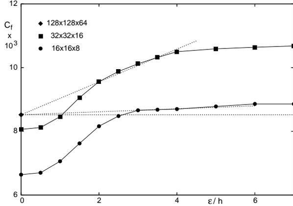
Figure 1: The skin friction coefficient as function of  $\epsilon/h$ . The results are computed with the help of the approximation  $C_4$ . The symbols represent the data at three different grids.
