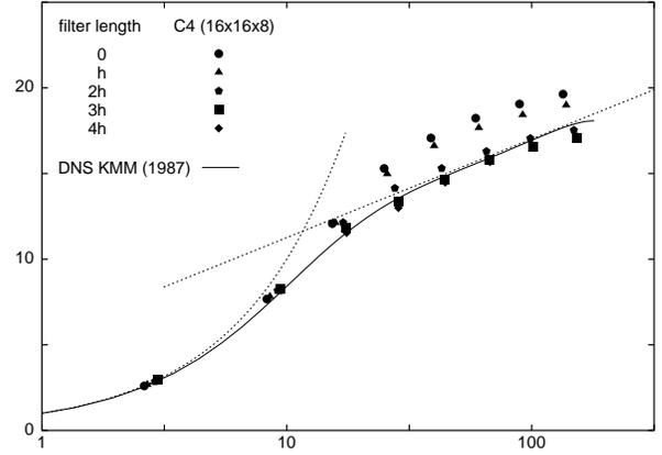
Figure 2: The mean velocity (in wall coordinates) as obtained from the  $16 \times 16 \times 8$  simulations. The filter length  $\epsilon$  varies from zero to four times the grid width  $h$ .
