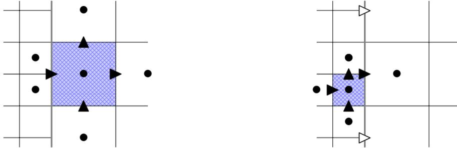
Figure 12: Visualization of the pressure Poisson stencil for the discretization given by (32). The velocity variables  $\blacktriangleright$  and  $\blacktriangle$  are used in  $M\mathbf{u}_h^{n+1}$ . The actual Poisson stencil for  $MGP_h^{n+1}$  consists of the pressure variables  $\bullet$ . Note that the variables  $\triangleright$  are only used on the right hand side in the term  $M^+\mathbf{u}_h^*$ .
