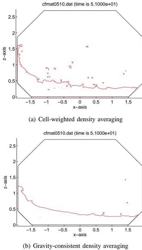
Fig. 4. Effect of the density averaging method on the free surface for a regular sway sloshing experiment with 10% filling ratio.
