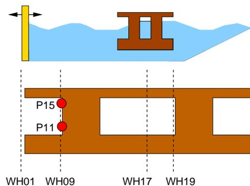
Fig. 8. Schematisation of the wave run-up test setup (top) and position of selected wave probes and pressure transducers (bottom).
