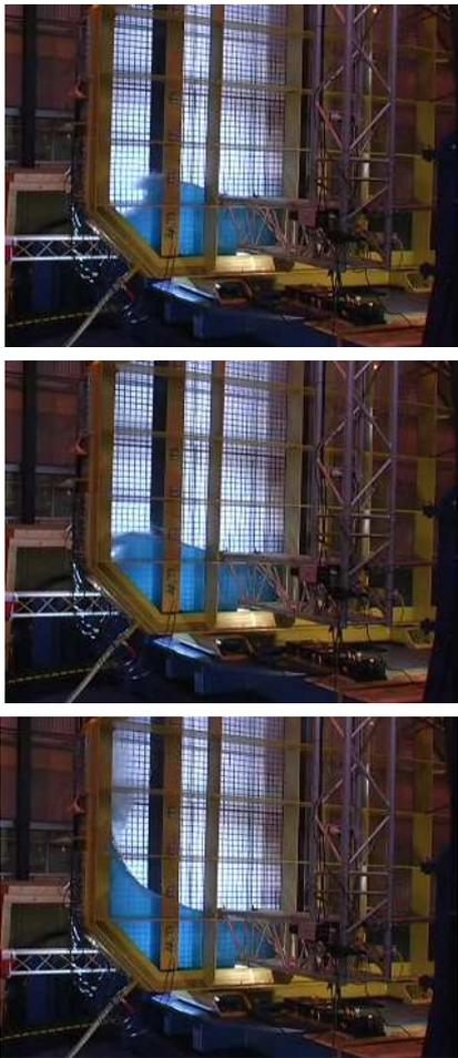
Fig. 6. Video frames of irregular 10% irregular sway and roll test around  $t = 140s$ : just prior, during and after air entrapment at the tank wall.
