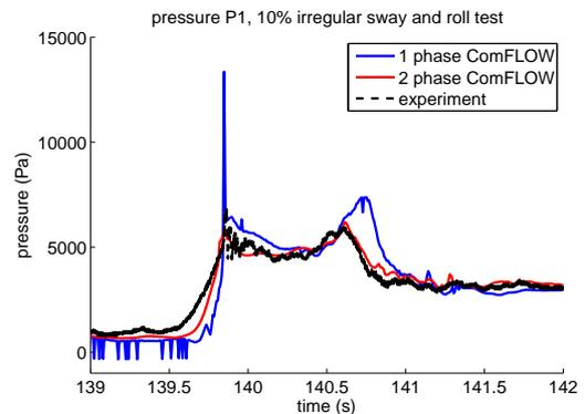
Fig. 7. Pressure development for transducer  $P01$  ( $x = 1.656m, z = 0.152m$ ) during the air entrapment case shown in Fig. 6.
