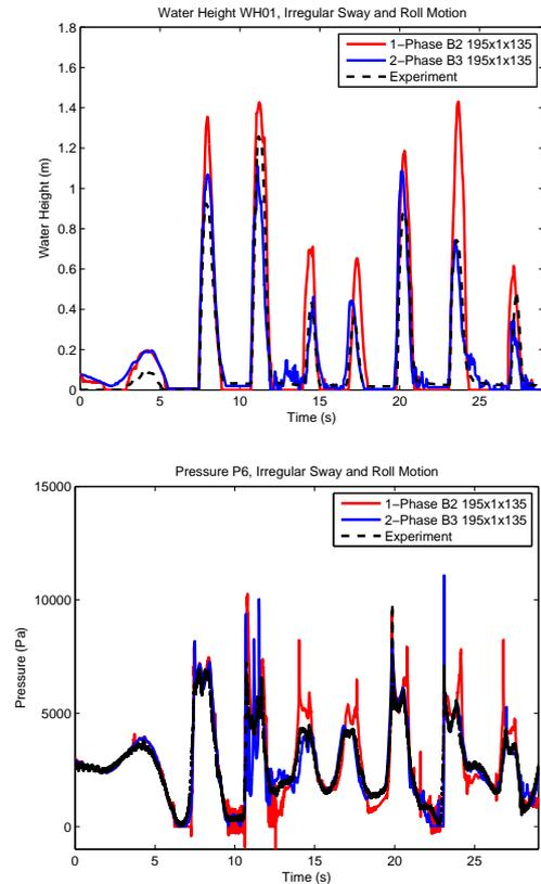
Fig. 5. Water height development for 10% filling ratio irregular sway and roll test at the tank wall (WH01,  $x = 1.89\text{m}$ ) and pressure signal at transducer P01 ( $x = 1.656\text{m}$ ,  $z = 0.152\text{m}$ ).
