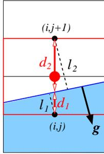
Fig. 2. Normal distances  $l_1$  and  $l_2$  and intersection distances  $d_1$  and  $d_2$  used in the gravity-consistent density averaging method.
