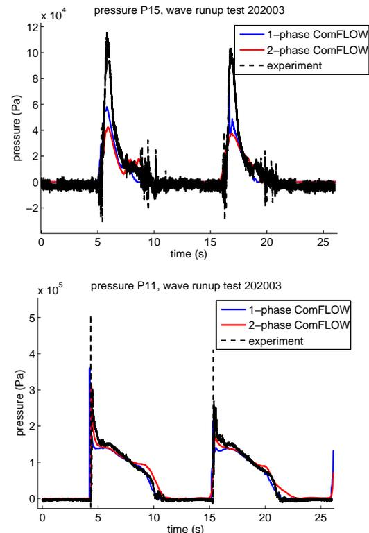
Fig. 11. Pressure development at the first column ( $x = -39.5m$ ): top ( $P15$ ) and bottom of the column ( $P11$ ).
