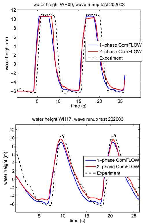
Fig. 10. Wave height development for run-up at the first column (WH09,  $x = -39.76m$ ), and wave height between the columns (WH17,  $x = 5.31m$ ).
