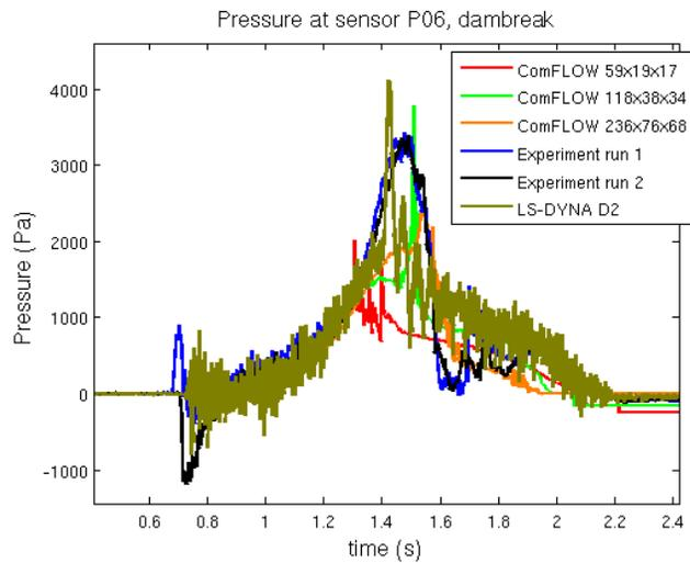
Figure 9 Pressure at vertical wall,  $z = 0.405$  m
