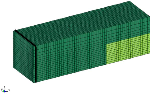
Figure 5 Positioning of rigid/elastic wall in LS-DYNA fluid domain
