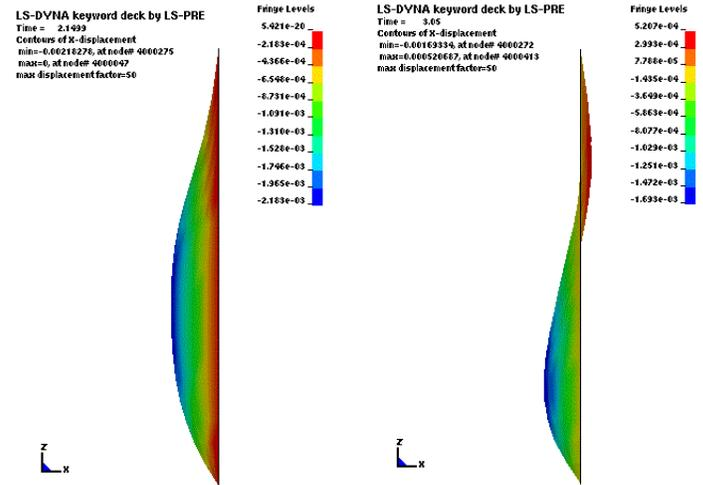
Figure 10 Deflection of flexible wall at initial impact,  $t = 2.15$  s (left), and after run-up against the wall,  $t = 3.05$  s (right).
