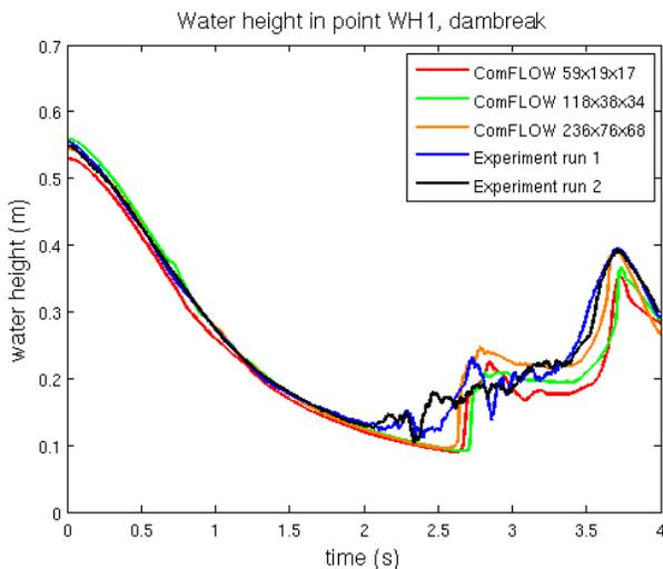
Figure 6 Water height in reservoir,  $x = 2.644 \text{ m}$
