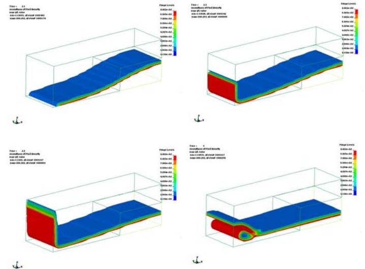
Figure 4 Three-dimensional snapshots of LS-DYNA simulation during wall impact.
