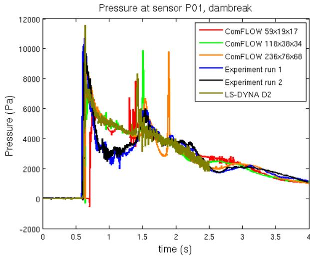
Figure 8 Pressure at vertical wall,  $z = 0.030$  m
