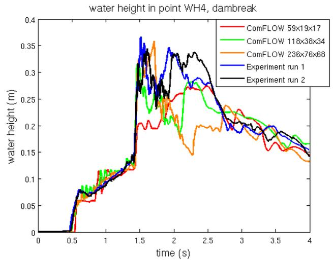
Figure 7 Water height close to left wall,  $x = 0.500 \text{ m}$
