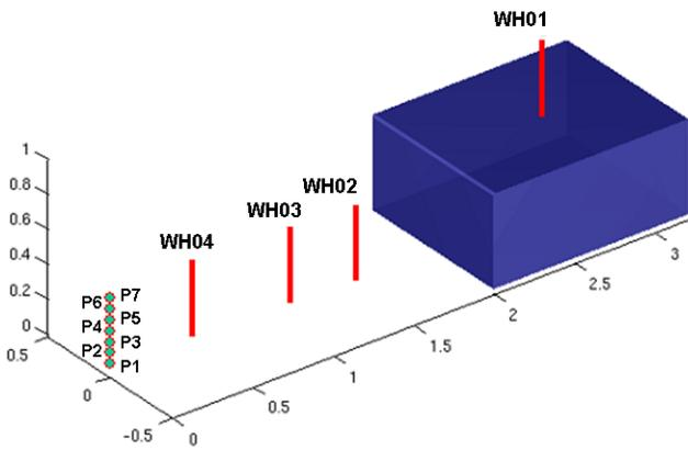
Figure 2 Positioning of wave probes and pressure sensors
