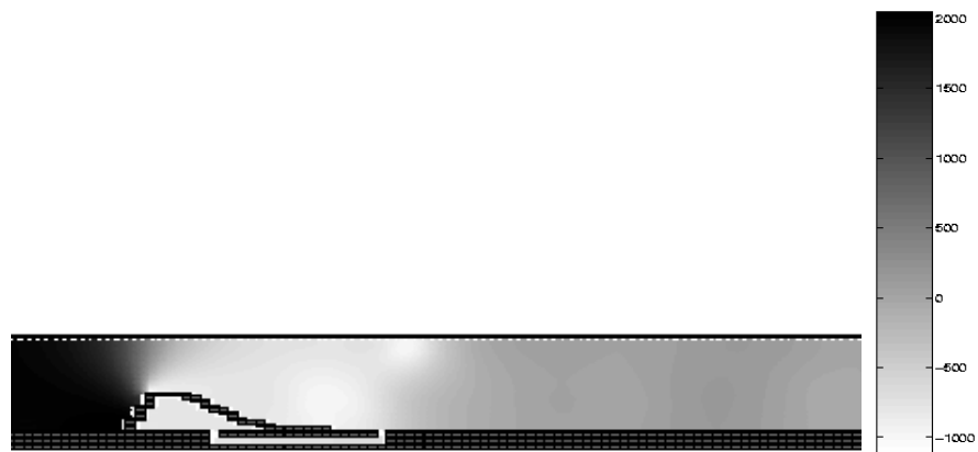
The pressure distribution when the lip collides with the lower wall.
