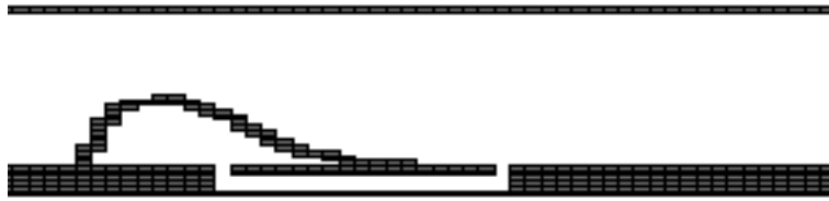
Figure 3.15: A pipe behind the base of the lip (pipe 1) is created in the model of Hamburg to prevent the enclosure of air.
