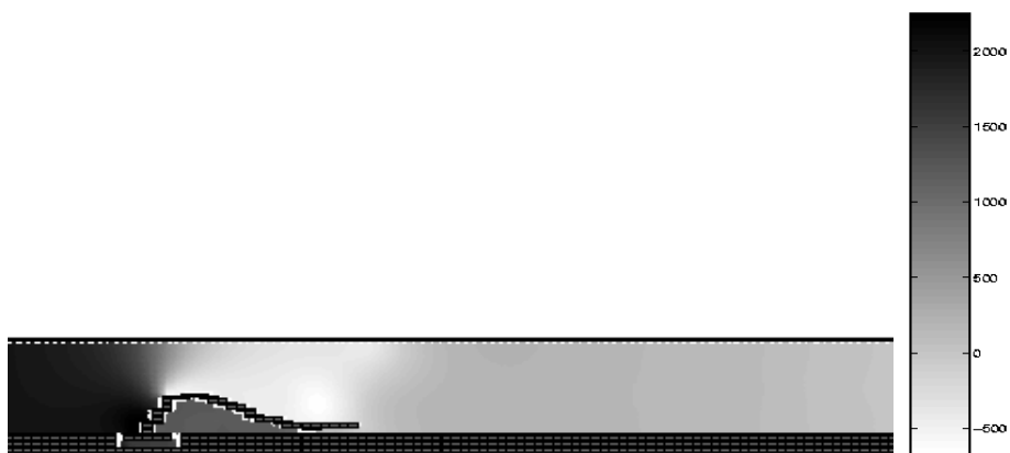
The pressure distribution when the lip almost collides with the lower wall.
