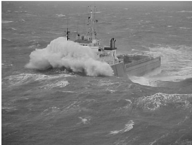
Figure 4.1: Green water smashing on a ship, accompanied by white water.
