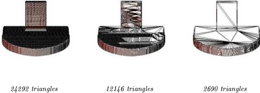
Figure 5.1: Decimation of the bow. The original triangulation of the iso-surface consisting of 24292 triangles is shown on the left. The middle figure is a reduction to half of the original number of triangles on the left (12146 triangles). On the right, with 2690 triangles the target reduction of polygons of 90% is only approximated and not completely accomplished due to the prevention of distortions. A further reduction can not be achieved without a violation of the original shape.
